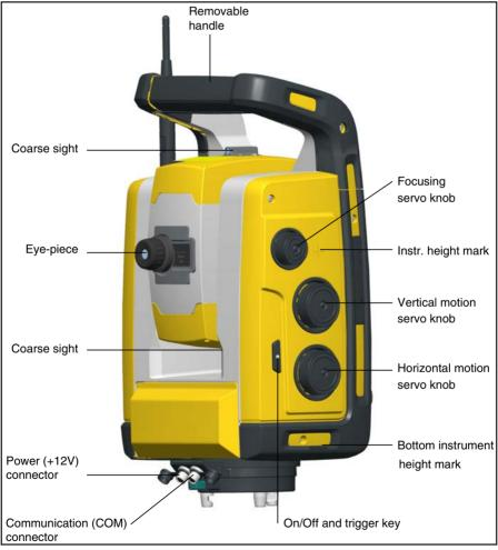
Figure 3.7 Operator's view of the Trimble SPSx20 Total Station
