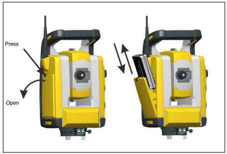
Figure 5.38 Removing and replacing the internal battery
